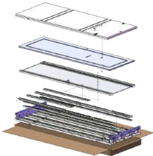
carton 2:frame+mounting profile+door+side panel carton 4:vertical management if needed
